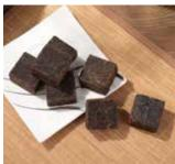
Crushed activated carbon, which raw material is more than one kind of selected bituminous coals, is made by the process of blending, powdering, briquetting and other steps.
